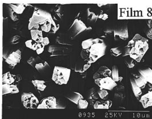
Figure 2. SEM graphs of the solution-grown films 4 , 7 , and 8 by varying the concentrations from 50, 10, to 5 mM in acetonitrile.
